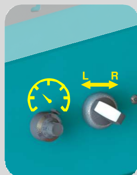
Adjustment of belt forward speed and direction
